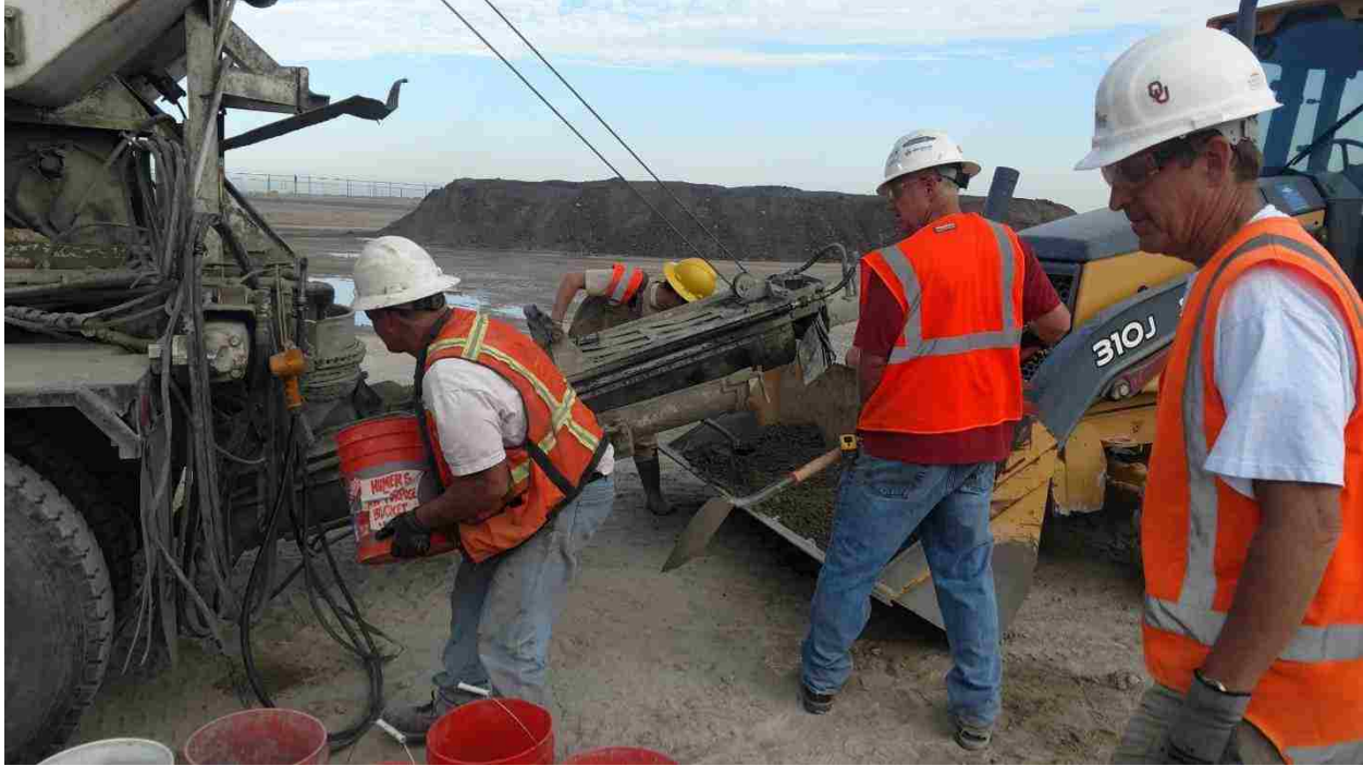
Figure 3-8. For 0° test, extra aggregate was added to each batch in order to meet cement content requirement.
